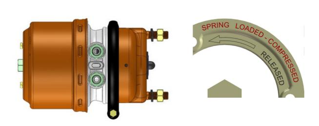
CONDITION: Spring Brake De-Activated (Spring Loaded - Compressed)
