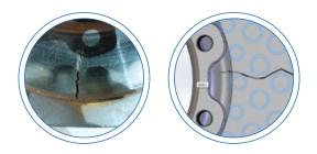
As a result, most failures of brake discs happen in the form of radial cracks or fractures. Vehicles mostly effected by thermal cracking are commercial vehicles including fire engines, motorway coaches, mountain buses and truck racing.
